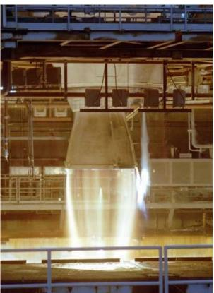
Figure 3. Delta IV First-Stage/RS-68 Engine Static Fire Test
