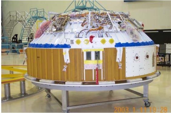
Figure 1. The Centaur Forward Adapter (CFA) is the structural basis for the DSS
