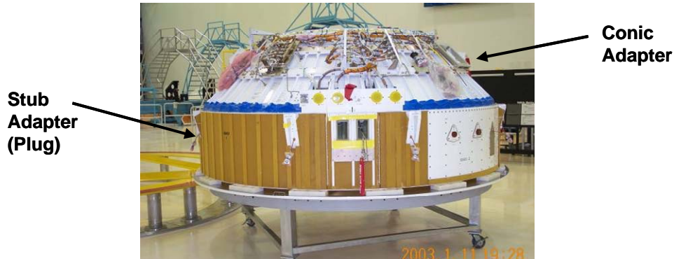
Figure I-1: The Centaur Forward Adapter (CFA) is the structural basis for the DSS
