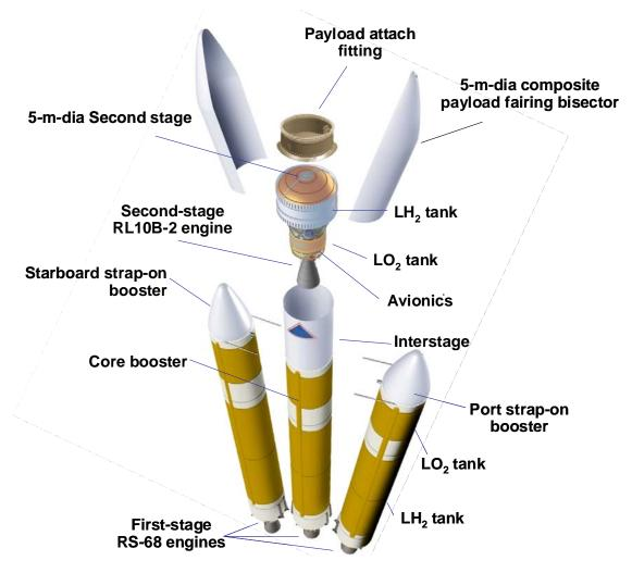
Fig. 4: First West Coast Heavy Vehicle Configuration
