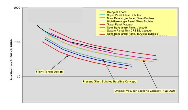
**Figure 5, Vacuum Insulation Panel Materials**
