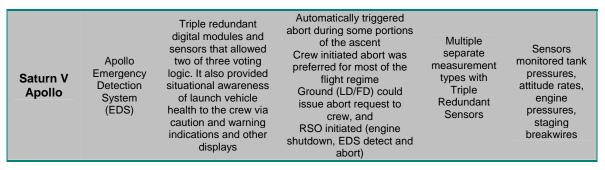
Figure 4: Launch Vehicle Health Monitoring schemes in previous Expendable LV Human Space Flight programs have focused on simplicity and reliability.
