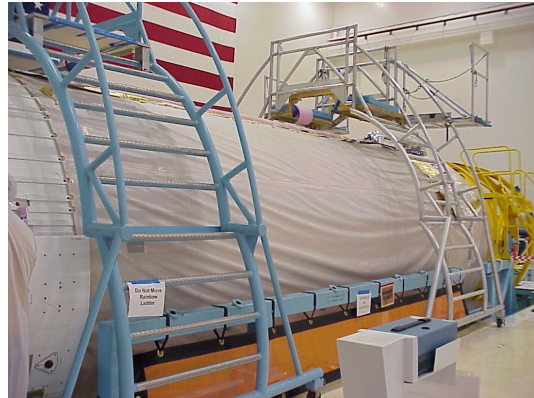
Figure 4. AV-005 During Final Assembly With Single-Layer Radiation Shield (that does Double Duty as a Foam Debris Shield) On Sidewall
