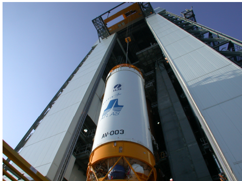
Figure 5. AV-003 Being Hoisted at the Vertical Integration Facility Showing the White Decal on Centaur Sidewalls.
