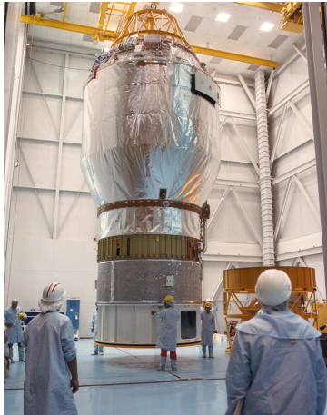
Figure 6. A G-Prime Centaur Tank in Clean Room Showing 3-Layer MLI on Centaur Sidewalls.
