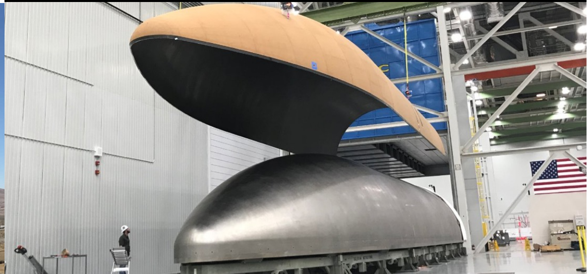
First Made-in-America Out of Autoclave Composite Payload Fairing
