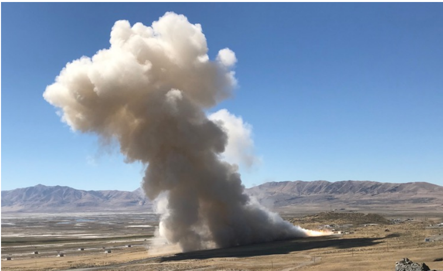
GEM 63 Static Test Fire
