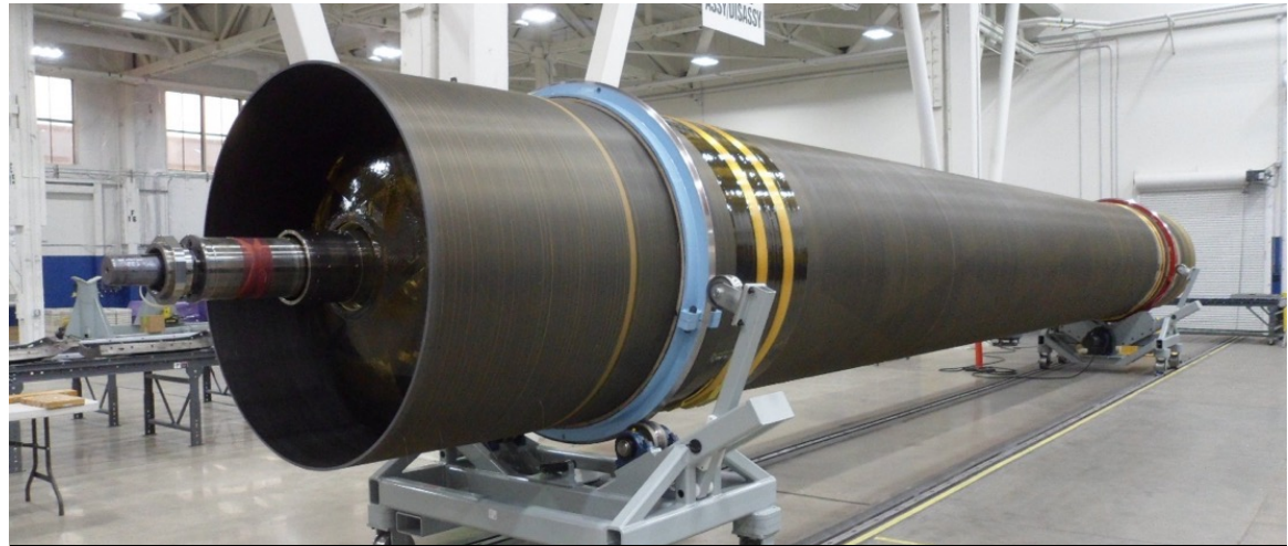
GEM 63 Structural Test Article Case Wind, Longest monolithic SRB case ever produced
