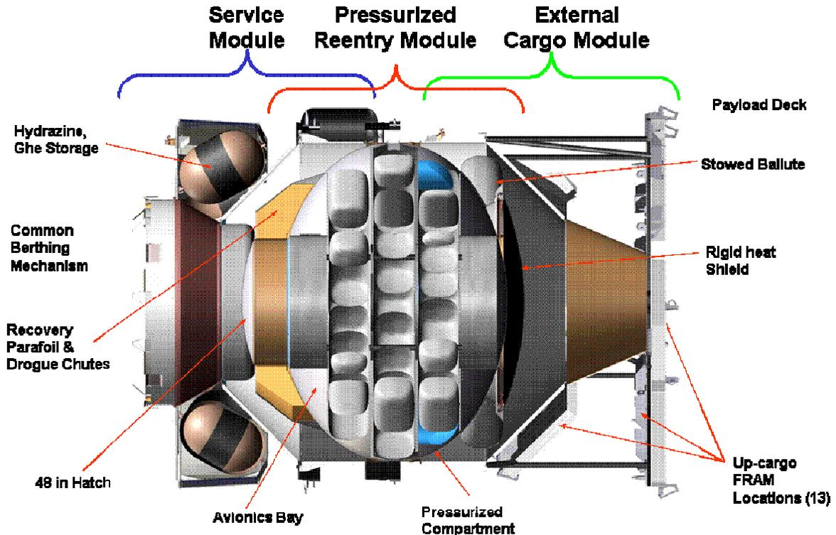
Figure 3. ARCTUS is composed of three primary elements, the external cargo module, pressurized reentry module, and the service module
