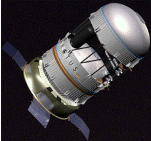
Figure 13. ARCTUS can support propellant resupply of orbiting fuel depots.
