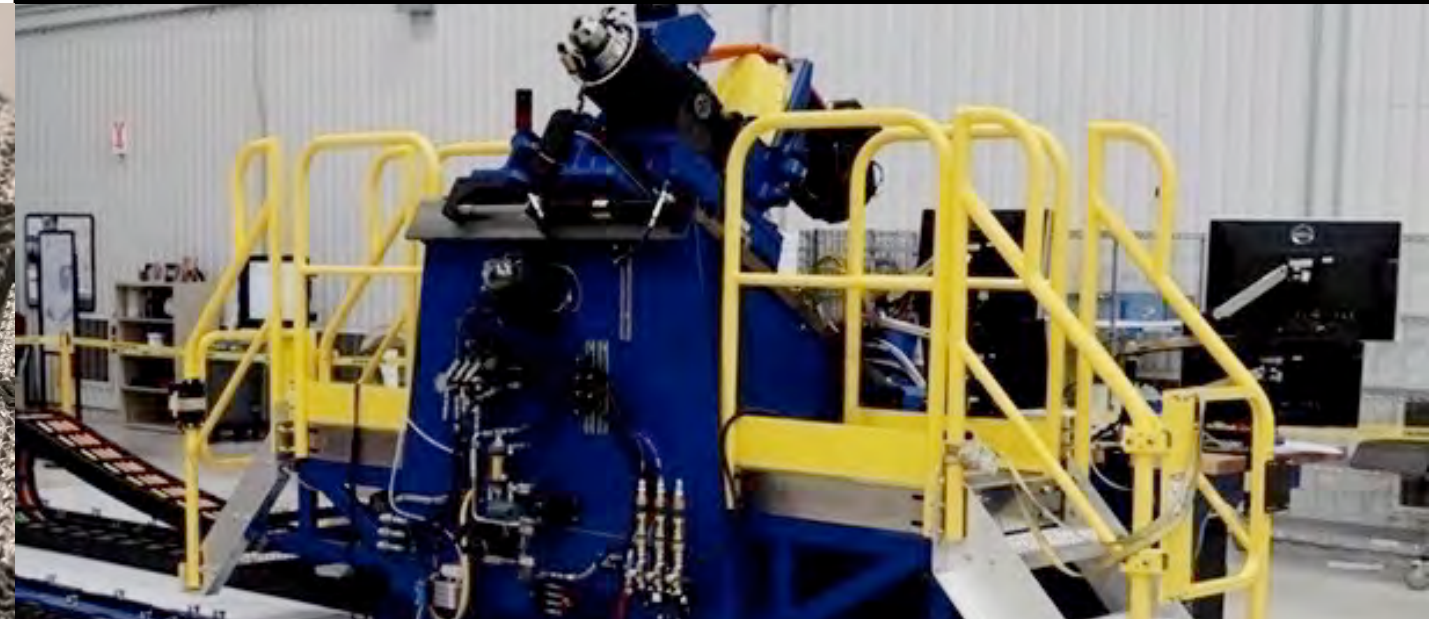
Circumferential Friction Stir Welding (CFSW)
