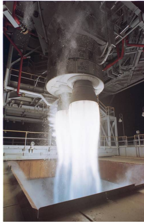
Figure 17 RD-180 Hot Fire
