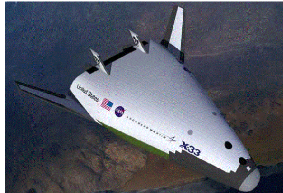
Figure 2 Fully reusable, single stage to orbit X-33 Concept pursued by Lockheed Martin and NASA, Credit NASA 2
