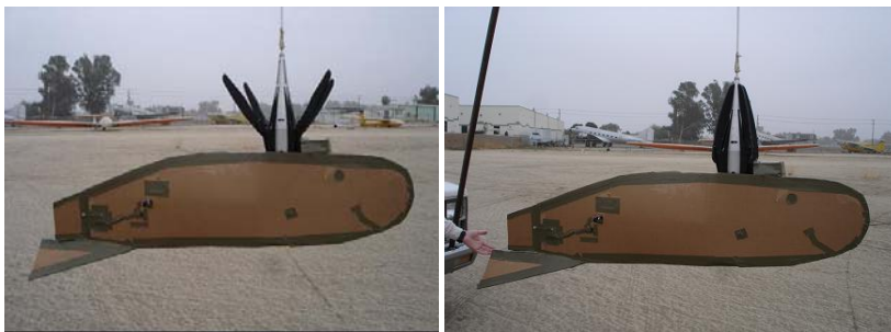
Figure 16 Grappling hook in open and closed positions
