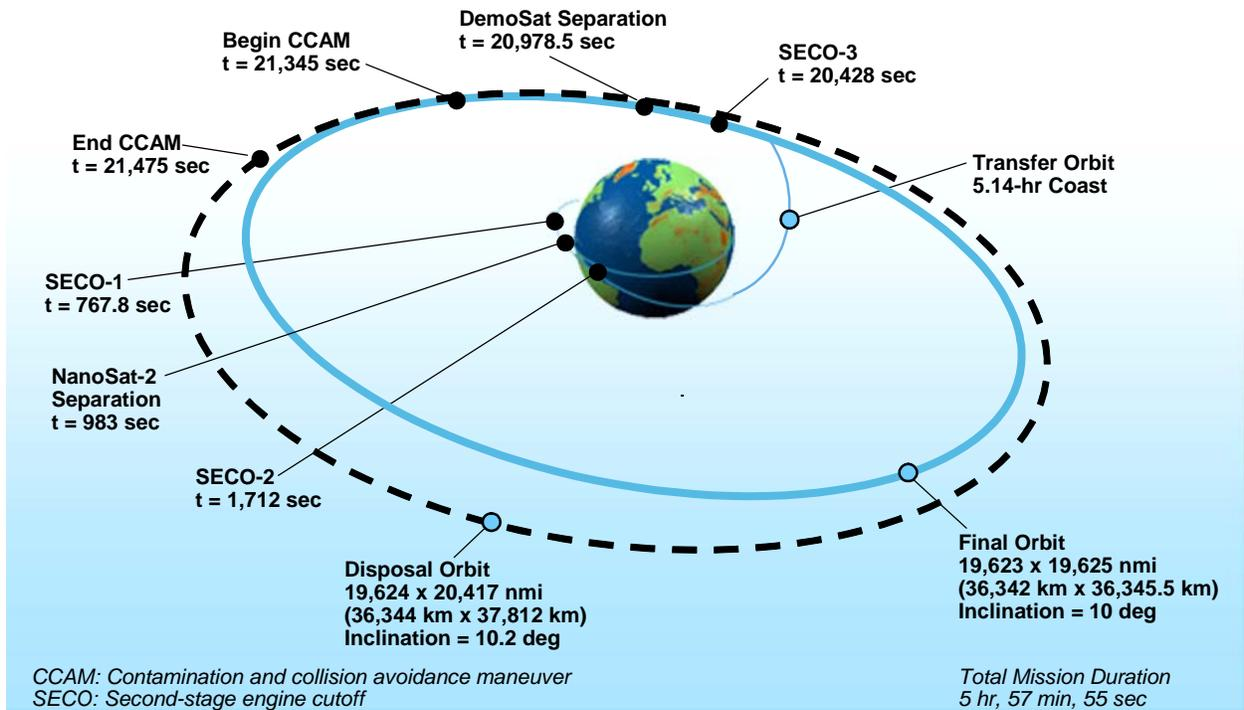
Figure 3. Delta IV Heavy Demo Orbit Planned Profile
