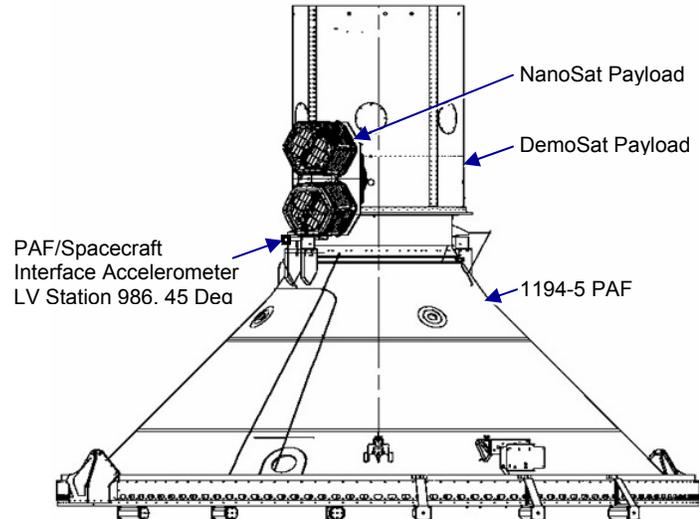
**Figure 12. Payload Attach Fitting Interface Accelerometer**
