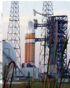
Vertical Placement of Vehicle on Pad
