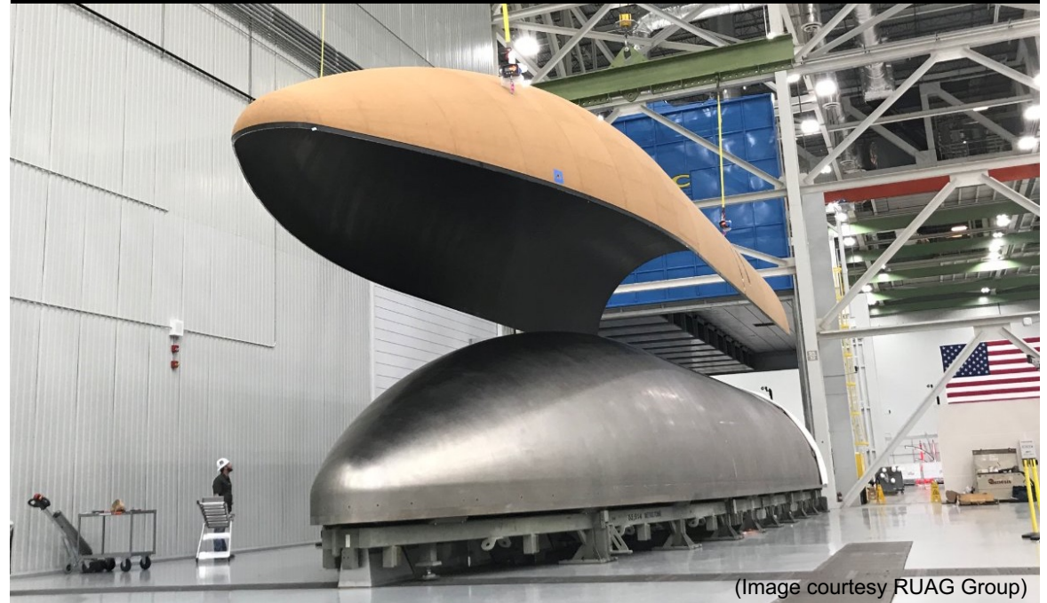
First Made-In-America Out of Autoclave Composite Payload Fairing
