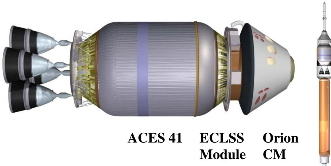
**Figure 3. ACES/Orion Vehicle Assembly.**
