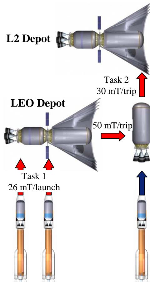
**Figure 8. A constant flow of propellant through the LEO depot to the L2 depot supplies the L2 depot and lunar operations.**
