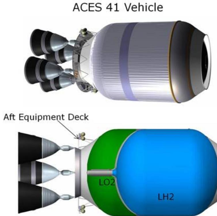
**Figure 2. ACES provides a light weight, thermally efficient propulsion system that can provide the foundation for all of explorations in-space transportation needs.**
