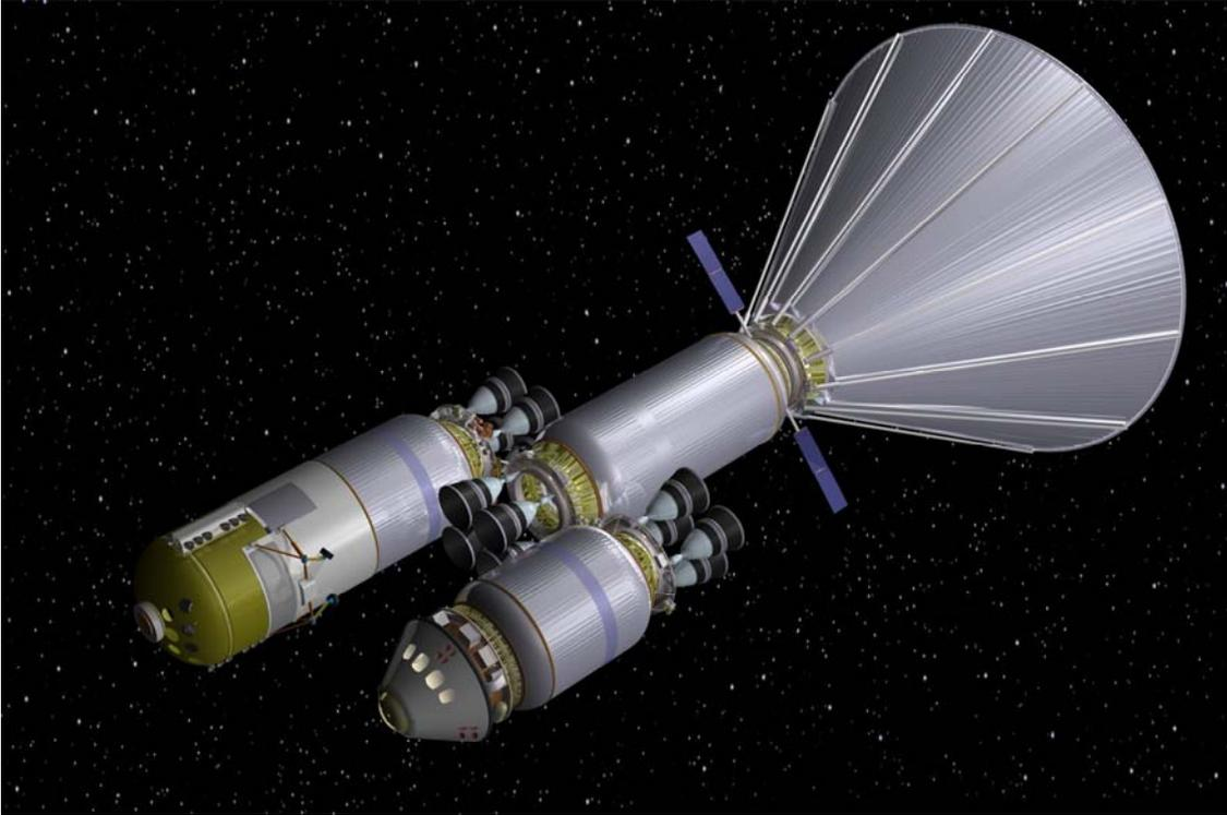
**Figure 7. L2 Depot with Orion and Altair Docked**
