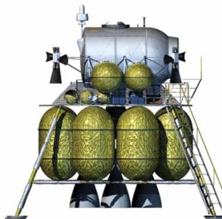
**Figure 3. Multiple LO<sub>2</sub> and LH<sub>2</sub> tanks complicate cryogenic fluid storage and handling while increasing weight and complexity of the baseline ESAS lunar lander. Image courtesy of John Frassanito & Associates.**
