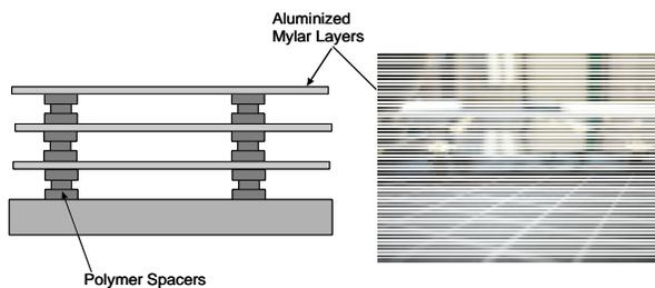
Figure 7 - Integrated MLI provides enhanced thermal and MMOD protection
