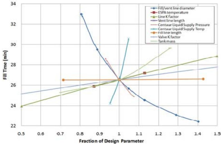
Figure 4 - Parametric analysis of CRYOTE tank cool down and fill design parameters
