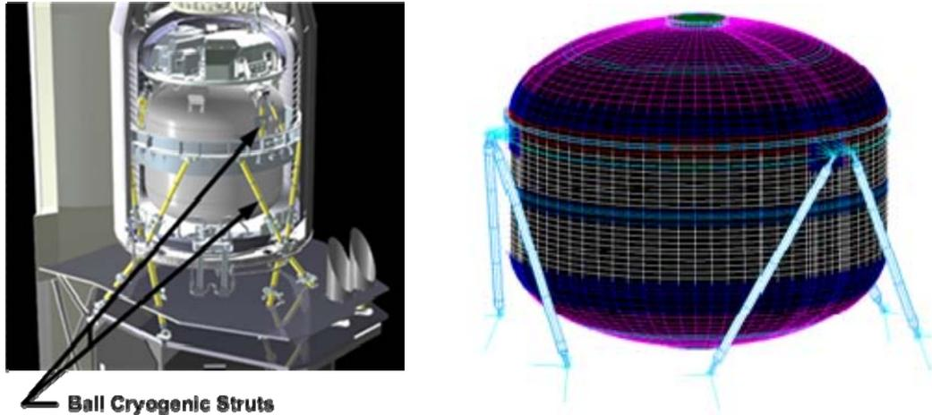
Figure 6 - Ball Aerospace flight heritage cryogenic strut technology has been optimized to meet the structural and thermal requirements of the CRYOTE missions
