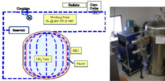
Figure 9 - NASA/Ball Aerospace Broad Area Cooling test program
