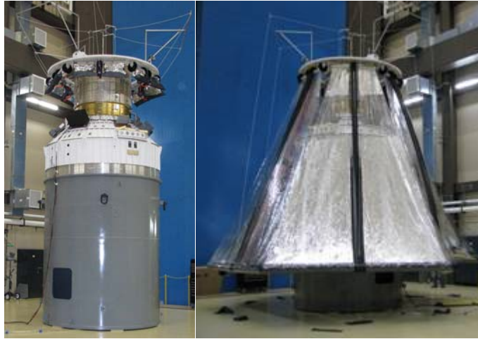
Figure 2: CSS 2007 Deployment Test; Stowed & Deployed Configurations
