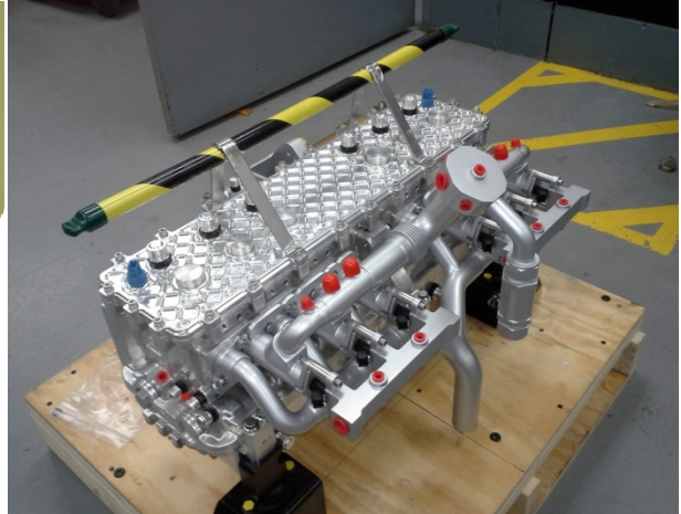
Figure 9 GH2/GO2 6 cylinder internal combustion engine developed by Roush has accumulated over 300 hours of successful run time.
