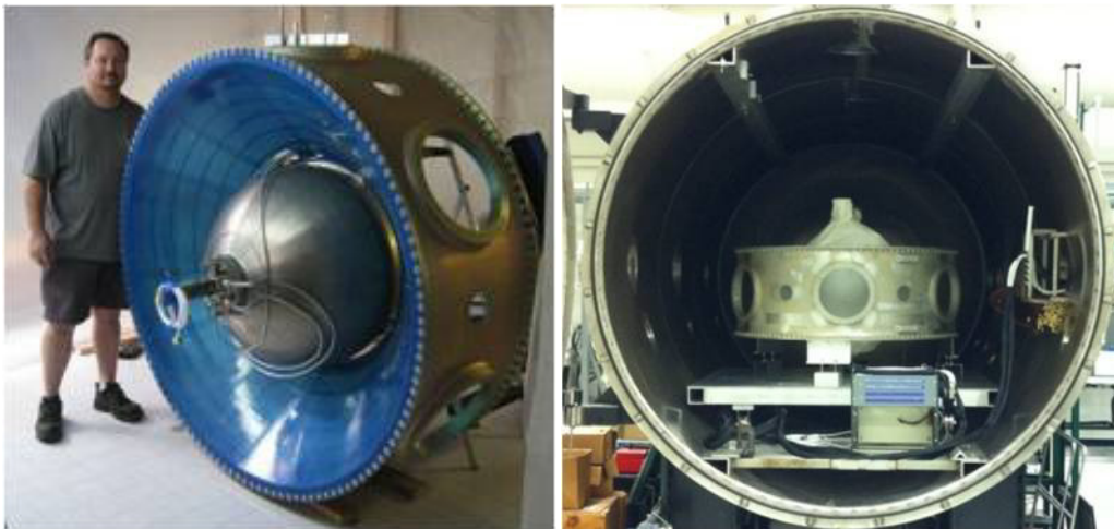
Figure 12 CRYOTE 1 provided affordable cryogenic storage testing of an integrated system.
