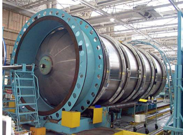
Figure 4 The Drop Tank, like Centaur's tank, will be produced from thin walled stainless steel resulting in a very light weight tank with low thermal conductivity for enhanced cryogenic storage.
