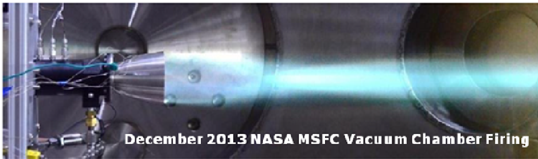
Figure 8 Testing IES's GH2/GO2 thruster in NASA MSFC's vacuum chamber.
