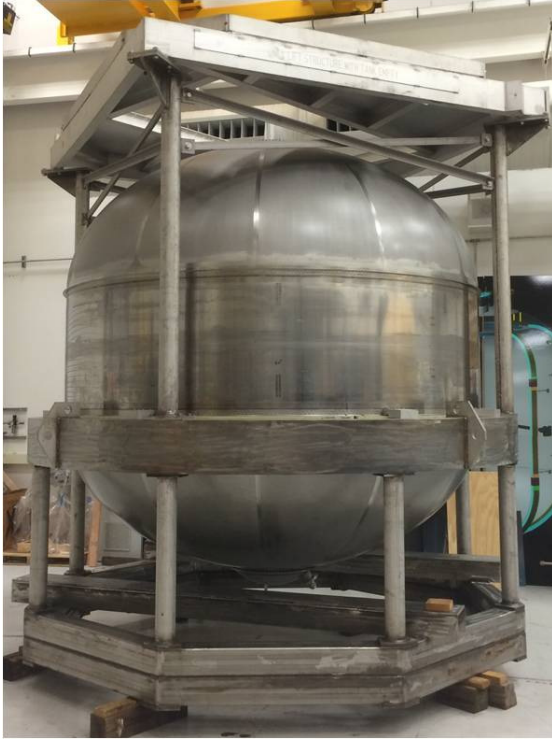
Figure 14 CRYOTE 3 is supported by a ring connected to the bottom tank flange, equivalent to the interstage adapter connecting the upper stage and booster or the Drop Tank truss adapter.
