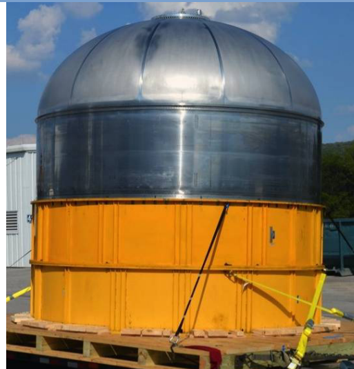
Figure 13 CRYOTE 3 is a 10 foot diameter, Centaur derived flight qualified tank designed to demonstrate high fidelity low boiloff cryogenic storage and transfer.
