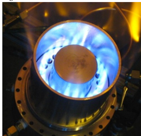
Figure 9 Axial Thruster Test
