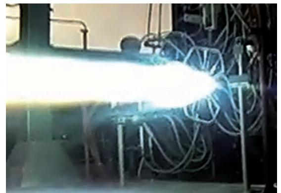
BE-4 staged combustion testing
