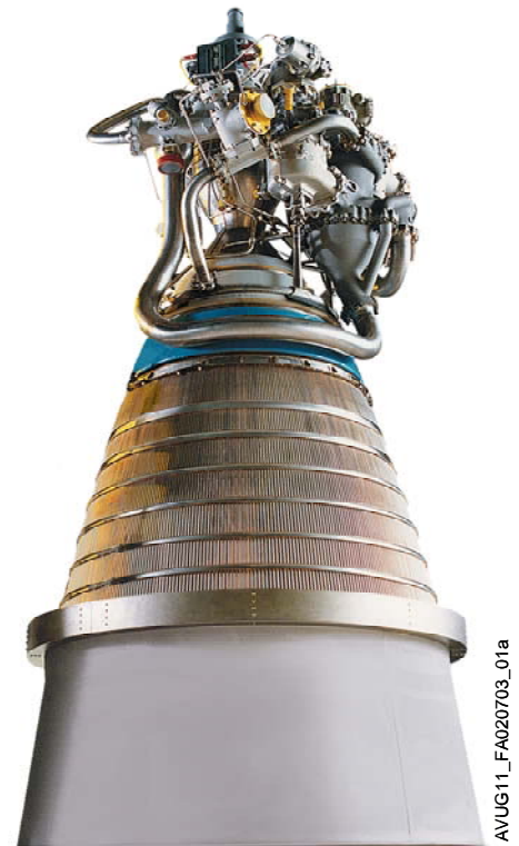
Figure A.2.7.3-1: RL10A-4-2 Engine
