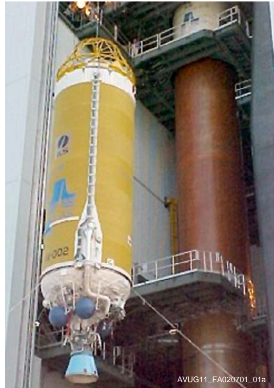
Figure A.2.7.1-1: Monocoque Centaur Tank
