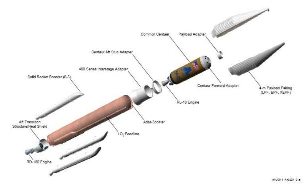
Figure 2 - Atlas V Launch Vehicle expanded view
