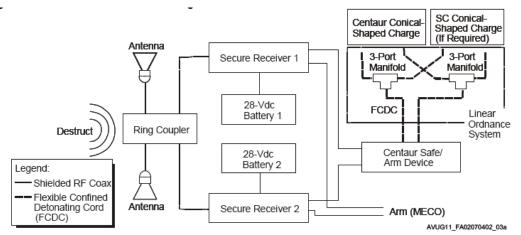
Figure 4 – Flight Termination System and Ordnance items
