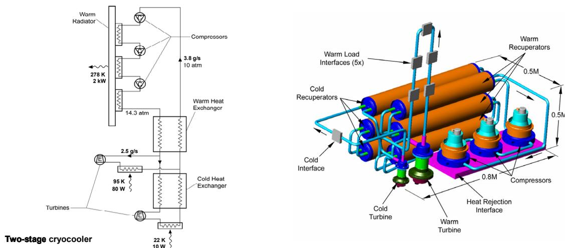
Figure 3-1. ACES Cryocooler Configuration and Layout
