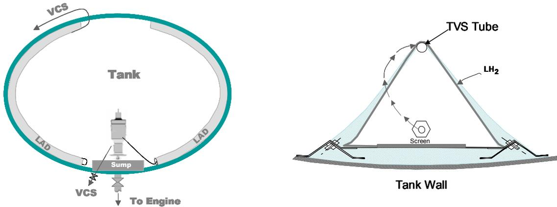
Figure 2-7. Thermodynamic Vent System (TVS) Schematic and LAD Configuration
