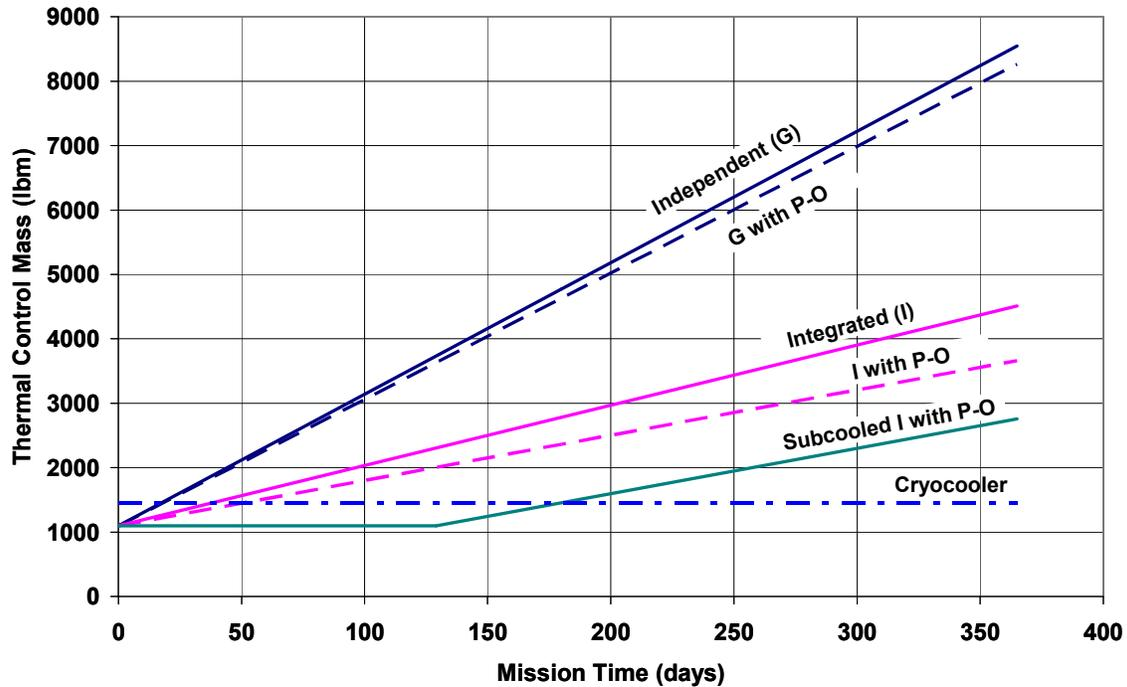
Figure 3-2. Boiloff Comparison Using Active Technologies
