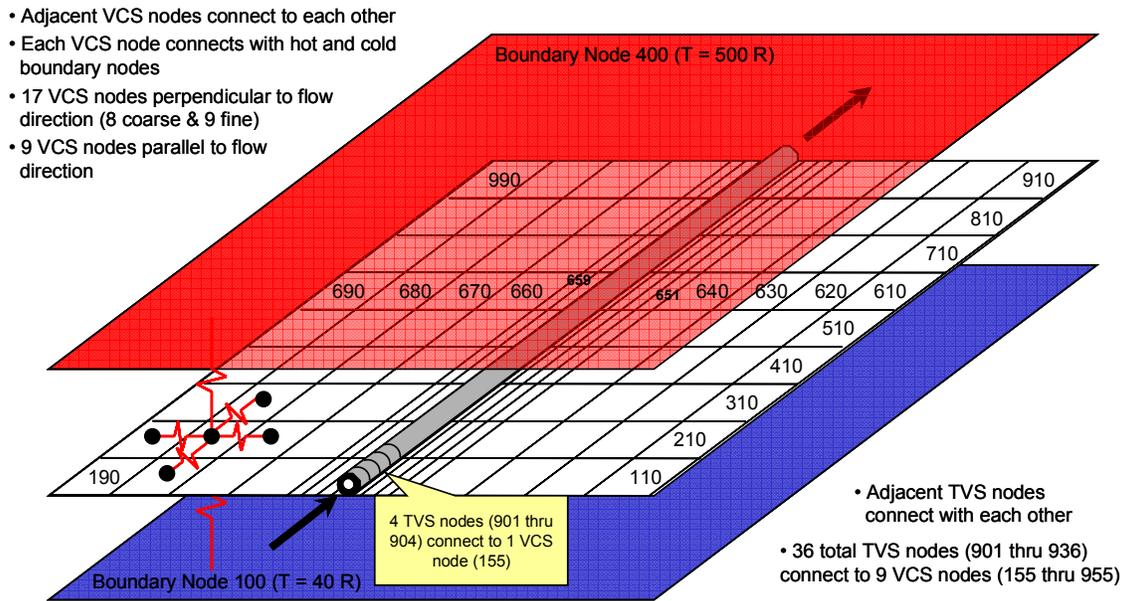
**Figure 2-6. Single Panel Isometric View**
