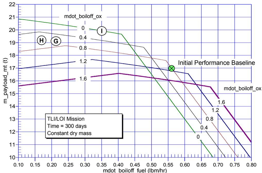
Figure 5-1. Effect of Boiloff on Payload (TLI/LOI-300 days)
